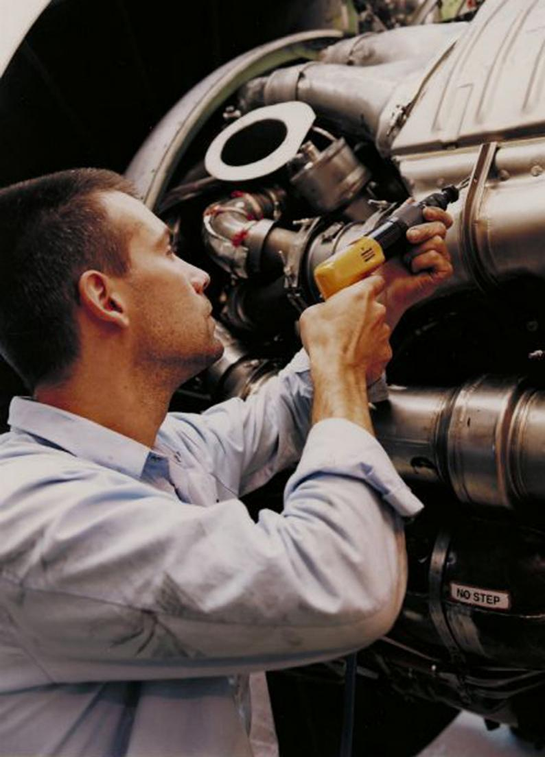
Atlas Copco tappers are designed for tapping and thread-cleaning operations with thread taps. The tools are fitted with a tap chuck as standard.
